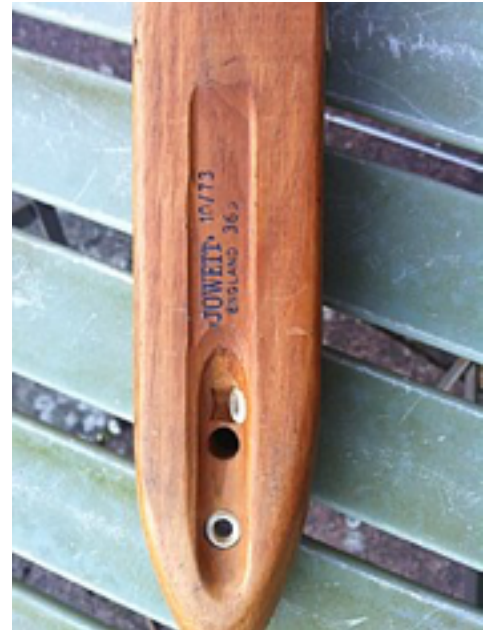
The bottom of the suction shuttle, manufactured and dated by Jowetts in 1973, showing the eyes
