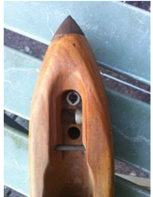
Three eyes are visible. Two lead through to the bottom, one leads to the side.
