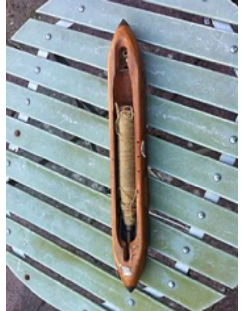
The top view of the shuttle shows the position of the pin and a number of ceramic ringed eyes leading to short tubes through the body of the shuttle.
