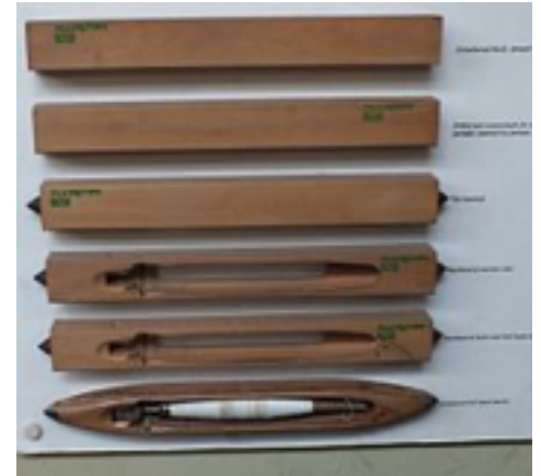
The stages in making a hand-threaded shuttle
